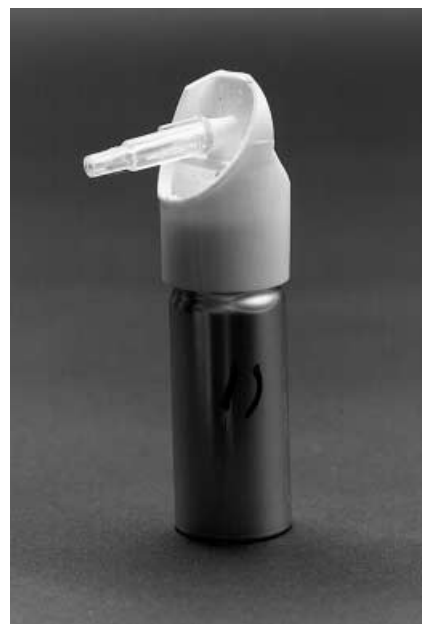
Fig. 1 Prototype of metered dose inhaler with modified adapter for use with the angiocatheters used for endotracheal intubation of the rat
